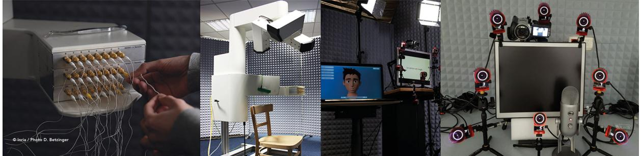
Figure 1: Multimodal Speech acquisition platform - Illustrating the articulograph, and the Motion capture system.
