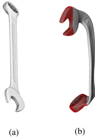
Figure 5: Tetrahedral mesh deformation, locked vertices are shown in red. (a): Shape, (b): our untangling result.
