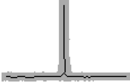
Figure 2. Position of the junction point with a skeleton-based method.
