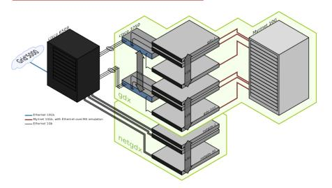
gdx @ Orsay: 18 24-ports switches connected to the main switch
