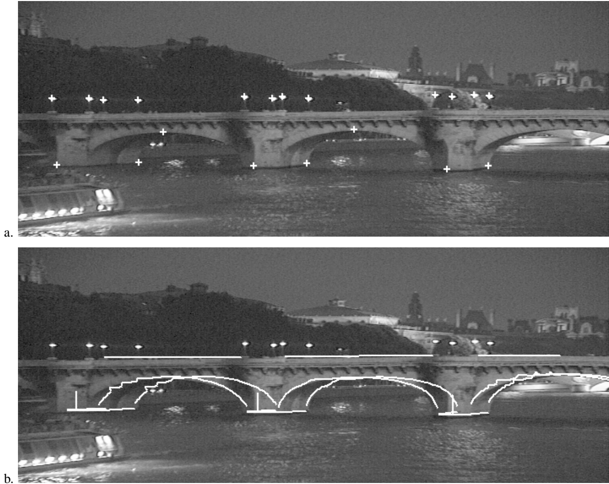
Figure 10: Matching 2D and 3D primitives. a. The first image of the sequence, including 20 points extracted manually from the contour map. b. Result of computing viewpoint by automatic 2D-3D primitive matching.
